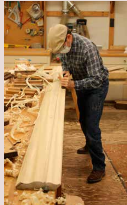
Craftsman C. J. Frost hand planes an entablature molding using antique plane, 2021
